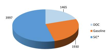
Total catalyst material for smelting/refining 7.392 t/year
